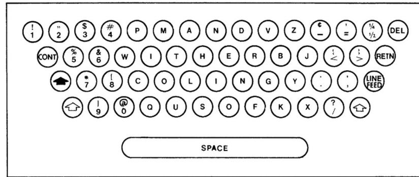
Figure 6: Montgomery's wipe-activated keyboard layout.
